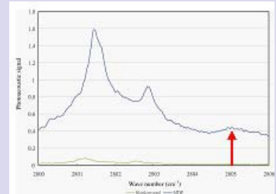
Figure 6. Measured photoacoustic spectrum of (a)LVL and (b)MDF formaldehyde emission in ambient laboratory air.
