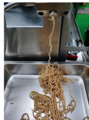
Fig 2 : The production process of bean noodles using extrusion technology.
