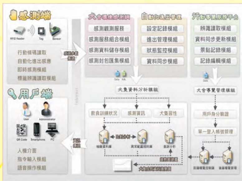
Fig.2 the system architecture of Livestock Health Management and Environmental Monitoring System.
