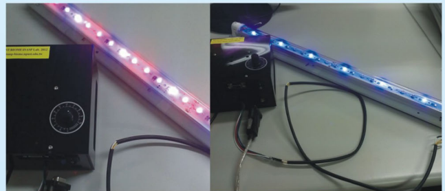
(c) The LED dimming control system
